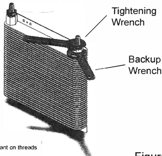
NOTE: Use thread lubricant on threads when installing fittings
