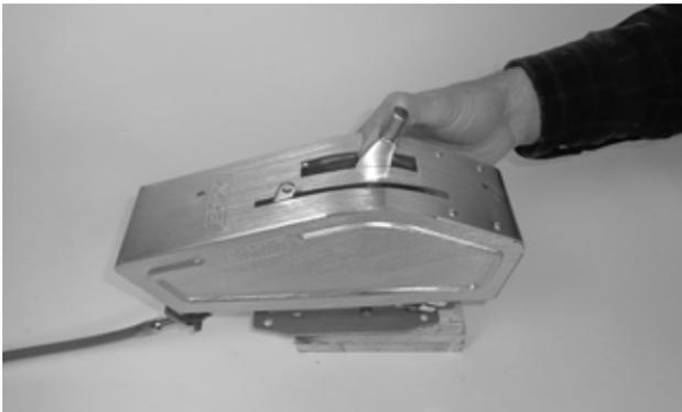
**B. Verify the shifter mechanism is free of any debris and hardware.** Lower the cover over the tips of the stick and the reverse lockout lever.
