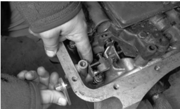
20. **Align and assemble the internal and external selector levers:** Hold the internal selector lever stationary, and rotate the selector shaft until its flat aligns with the serrations on the internal lever's pinch clamp. Push the shaft firmly into the transmission until the internal lever stops against the shaft's shoulder, then tighten the pinch bolt.
