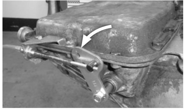
**31. With the swivel still in the selector lever, pull the shifter back to LOW (position 6),** verifying that the swivel slips freely in and out of the **B&M 1** hole in each position.
