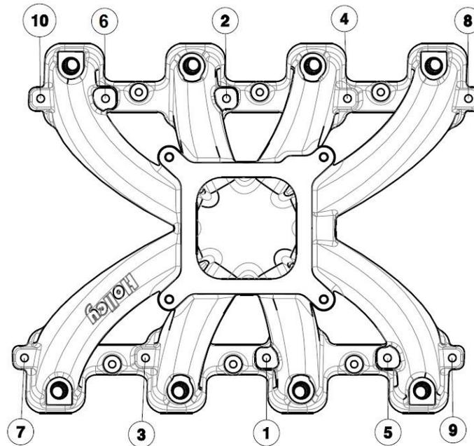
**Manifold Tightening Sequence**
