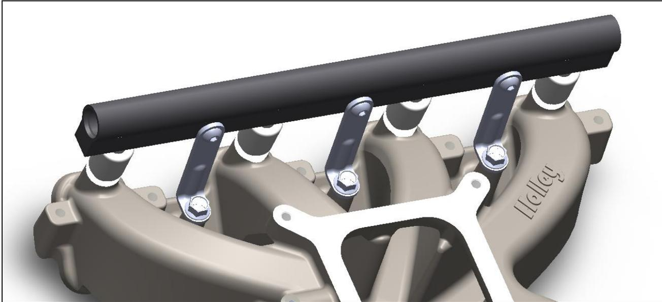
4. Tighten the mounting fasteners in two steps, 7 ft-lbs for the first step and 12-15 ft-lbs for the second step.
