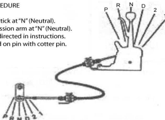
With shifter mounted in the desired location, direct eyelet end of shifter cable through shifter frame. Secure shifter cable to frame using cable clip, push clip down until it is firmly seated. Put shifter in neutral and slide cable eyelet over pin on shifter stick (see exploded view), install cotter pin (p/n 1900001) through hole in shifter pin to hold cable in place.
