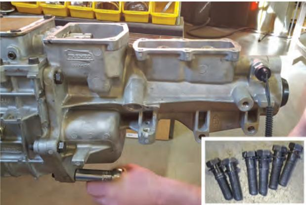
8. Remove (x6) bolts holding tail shaft housing on transmission.
