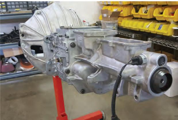
15. Re-install bolts (removed step 8) to secure tail shaft housing as shown.
