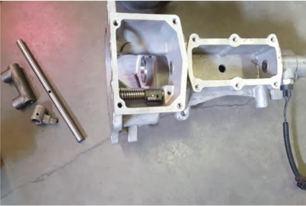
13. Remove double socket cup then set all parts aside. Make sure to remove roll pin (removed step 10) from the inside of tail shaft housing.
