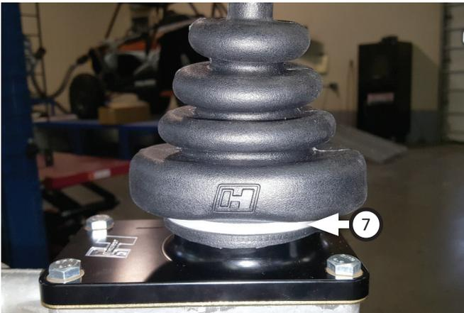
10. Install **dust boot (2)** over the shift stick and slide down onto the tower. Secure to tower with **zip-tie (7)**.
