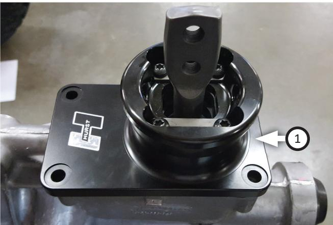
6. Guide shift rod ball into cup and place **shifter (1)** on pad.
