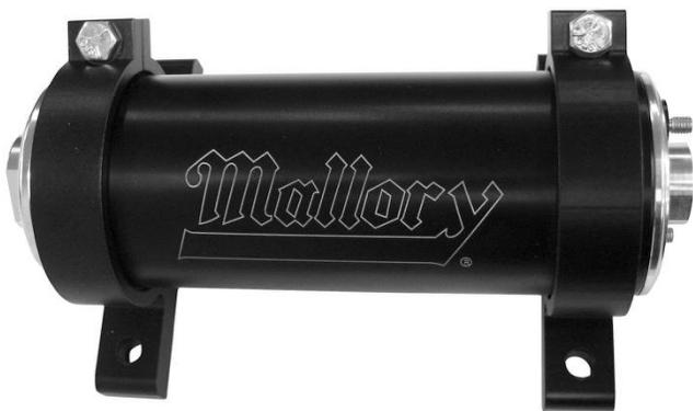
← When installing the pump, do not over tighten the nuts on the electrical posts. These need to be a **snug fit only**. Over tightening these connections can result in damaging internal connections and create a no run condition. This is considered damage at installation and not warrantied.
