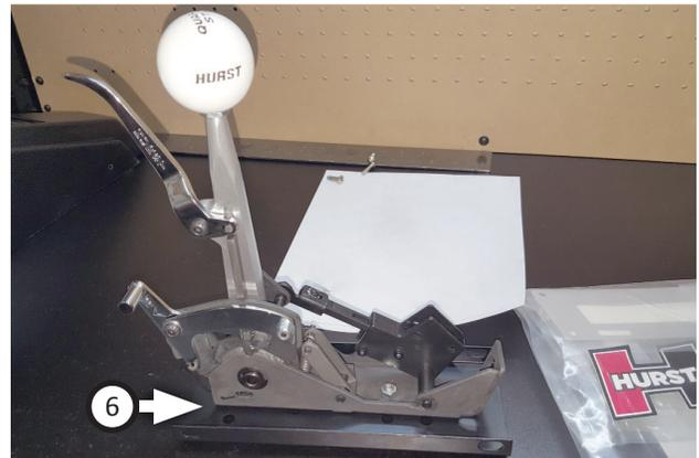
5. Place **console mounting plate (6)** under shifter frame and attach assembly to floor tunnel using same mounting holes securing shifter to floor tunnel. Fasten using (x4 ea.) **screws (8)** and **flat washers (9)**.
