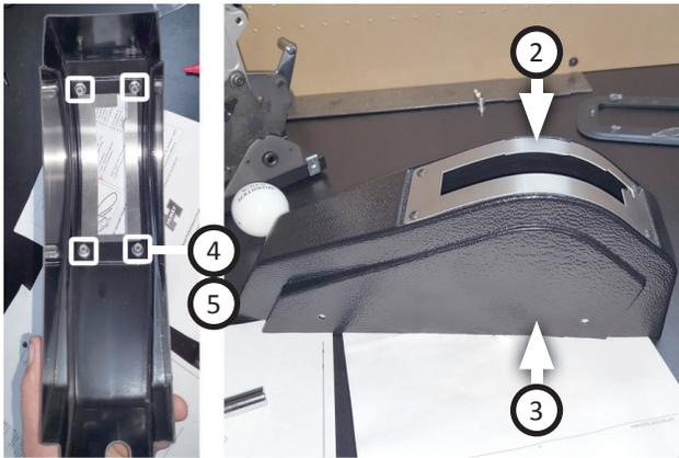
8. Place **gear indicator plate (2)** onto console, with slot for reverse lockout lever on driver side. Fasten forward portion of plate and console with (x2 ea.) **screws (1)**, **flat washers (4)** and **nuts (5)**.
