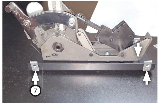
6. Install (x4) **u-shaped nuts (7)** onto both sides of mounting plate (extruded side toward inside of plate).
